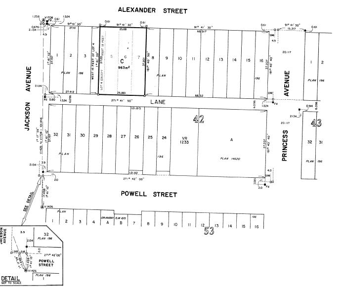
INTEGRATED SURVEY AREA NO. 31 CITY OF VANCOUVER. THIS PLAN SHOWS GROUND-LEVEL MEASURED DISTANCES. PRIOR TO COMPUTATION OF U.T.M. CO-ORDINATES, MULTIPLY BY COMBINED FACTOR OF 0.9995899737.
